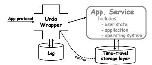
**Figure 1: Basic undo architecture.** The application service is wrapped with an undo layer that interposes on the verb-based application protocol, logging the intent of user changes for later replay. The undo wrapper also manages a time-travel storage layer used to implement rewind, and tracks state externalization to manage undo-induced inconsistency.
