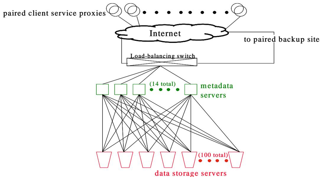
Figure 2: The architecture of one site of *Content*. Stateless metadata servers provide file metadata and route requests to the appropriate data storage servers. Persistent state is stored on commodity PC-based storage servers and is accessed via a custom protocol over UDP. Each cluster is connected to its twin backup site via the Internet.
