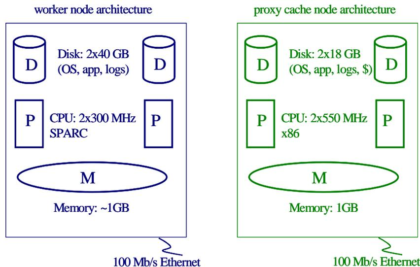
Figure 4: Architecture of worker nodes and proxy cache nodes in *Online*. Nodes contain two disks, two CPUs (SPARC in the case of worker nodes, x86 in the case of proxy cache nodes), about 1 GB of memory, and a 100 Mb/s Ethernet interface.
