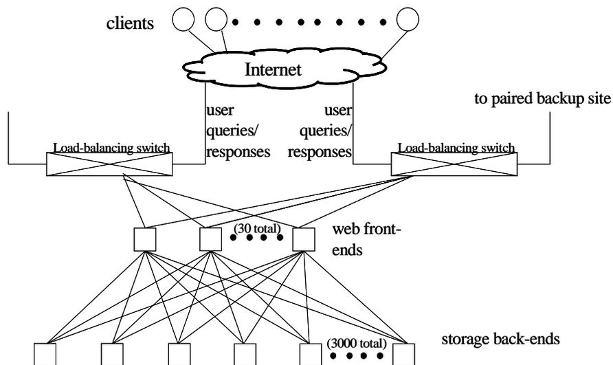
Figure 3: The architecture of one site of *ReadMostly*. A small number of web front-ends direct requests to the appropriate back-end storage servers. Persistent state is stored on commodity PC-based storage servers and is accessed via a custom protocol over TCP. A redundant pair of network switches connects the cluster to the Internet and to a twin backup site via a leased network connection.
