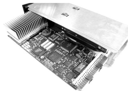
Fig. 2. An ROC-1 brick. The processor board is shown partially removed from the canister and with its disk removed.
