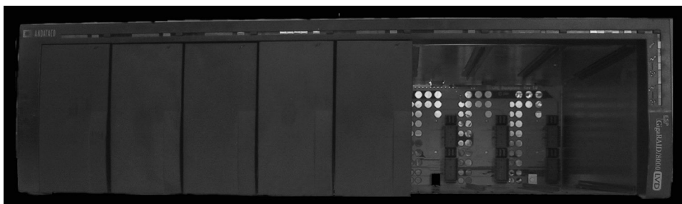
Fig. 5. A shelf with five bricks inserted and three empty slots.
