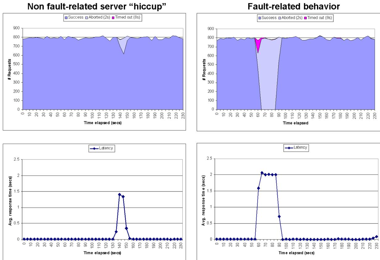
**Figure 9: A comparison of the throughput components and latencies of an HA-PRESS system during a spontaneous “hiccup” caused by resource exhaustion and an actual fault.** Note that the response times reach the connection abort time limit of two seconds during the actual failure, resulting in a 30-second interval during which all client requests either abort or time out. The service disruption that the spontaneous “hiccup” causes is comparatively minor.
